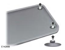
To install the floor mats, position the floor mat eyelet over the retention post and press down to lock in position.
