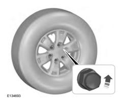
5. Remove the wheel nuts and the road wheel.
