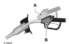
4. Hold the fuel pump nozzle in position B when refueling. Holding the fuel pump nozzle in position A can affect the flow of fuel and shut off the fuel pump nozzle before the fuel tank is full.
