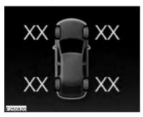
The tire pressure monitoring system measures pressure in your road tires and sends the tire pressure readings to your vehicle. You can view the tire pressure readings through the information display. See **General Information** (page 95). The low tire pressure warning light will turn on if the tire pressure is significantly low. Once
