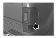
The sensors are inside the tail lamp on both sides of your vehicle.
