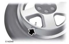
**Note:** Each road tire is equipped with a tire pressure sensor located inside the wheel and tire assembly cavity. The pressure sensor is attached to the valve stem. The pressure sensor is covered by the tire and is not visible unless the tire is removed. Take care when changing the tire to avoid
