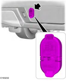
When attaching the trailer wiring connector to your vehicle, only use a proper fitting connector that works with the vehicle and trailer functions. Some seven-position connectors may have the SAE J2863 logo, which confirms that it is the proper wiring connector and works correctly with your vehicle.
