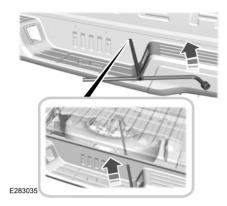
2. Insert the jack handle into the guide hole. Turn counterclockwise until the wheel rests on the ground, and there is slack in the cable.
