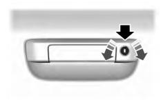
Insert the ignition key into the tailgate lock. Turn it to the left to lock the tailgate. Turn it to the right to unlock the tailgate.
