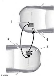
Connect the positive (+) jumper cable to the positive (+) terminal of the discharged battery.
