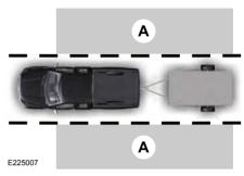
The blind spot information system with trailer tow is designed to aid you in detecting vehicles that may have entered the detection area zone (A). The detection area is on both sides of your vehicle and trailer, extending rearward from the exterior mirrors to the end of your trailer. When you attach a trailer and have set up a blind spot trailer, the blind spot information system with trailer tow becomes active when driving forward above 6 mph (10 km/h).
