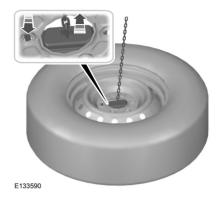
3. Pass the bracket and cable through the wheel opening.
