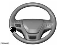
The adaptive cruise controls are on the steering wheel.
