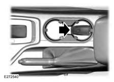
Place the passive key in the position shown, with the buttons facing upward. Make sure that you place the key fob in the center of the cup holder.
