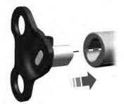
Remove the tailgate from the left-hand side hinge by sliding it to the right.
