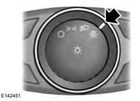
When the lighting control is in the autolamps position, the headlamps turn on in low light situations, or when the wipers turn on.
