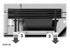
vehicle, rotate the lead screw of the jack counterclockwise to collapse the jack height. Ensure that jack is not fully closed.
