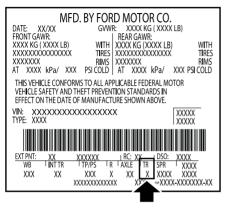
The transmission code is on the Safety Compliance Certification Label. The following table shows the transmission code along with the transmission description.
